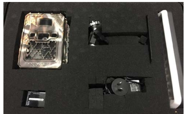
Photo: Monitoring Kit (including camera, bracket/band for installing, battery charger, card reader)
